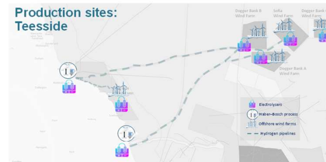
Figure 1. UK North Sea offshore wind-hydrogen system configuration. The map shows offshore wind developments across three corridors connecting to St Fergus, Bridlington, and Middlesbrough. Marine transportation routes (dashed blue) indicate seaborne transport pathways. Marine pipelines and transmission cables (dotted blue) represent subsea infrastructure. Inland hydrogen pipelines (dashed orange) connect hubs to Milford Haven. Insets detail production sites near St Fergus (floating platforms) and Teesside (fixed foundations). Symbols indicate electrolysers (purple), and offshore wind farms (grey turbines)
